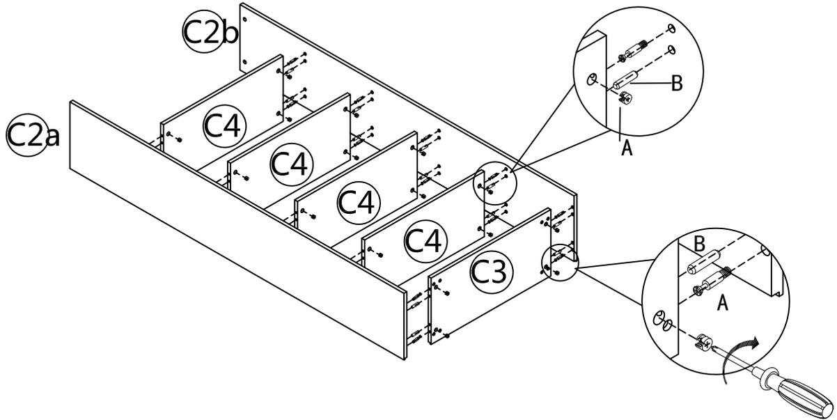
**STEP 2:** Insert the Dowel(B) to the Side Panel(C2a,C2b),Use a Phillips Head Screwdriver to insert the Cam Pin(A) to the Top Panel(C1),Assemble the Top Panel(C1) to the Side Panel(C2a,C2b),Use a Phillips Head Screwdriver to turn the Cam Lock(A)to lock onto the head of Cam Pin(A),Use Hex Key(F) to tighten the Leg(L)to the Bottom Panel(C3) with Bolt(C).
